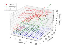
Figure 1: LCI outperforms MPICH and OpenMPI on OpenMP using multi-threaded point-to-point varying number of sender or receiver threads. Performance is done on Stampede2 cluster.
