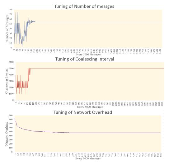
Figure 1: Tuning the number of message in a parcel and coalescing interval and its impact on network overhead
