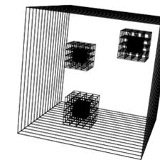
Test case with 3 spherical charges, adaptive grids shown above.
