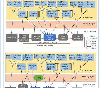
2 Holistic workflow diagrams of DroughtHPC: Files accessed in simulation of a single cell, with multiple meteorological data (Number of samples), and time period (Number of days). Gray sections refer to Python code, and blue refers to the hydrologic model . Top: VIC accesses 57 files in total in each call. Bottom: Hydrologic model (VIC) code is changed to minimize forcing data's movement between storage layers, and reduce invocation cost
