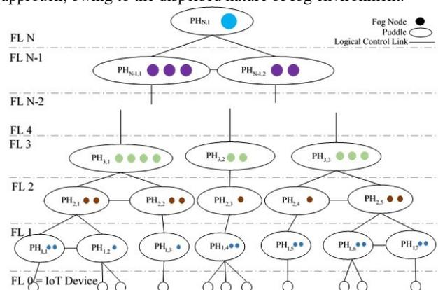
**Figure 1: Logical organization of heterogeneous fog nodes into multi-layered hierarchy.**
